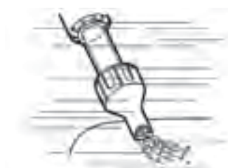
Double function nozzle: specially designed for debris at the bottom and corners.
